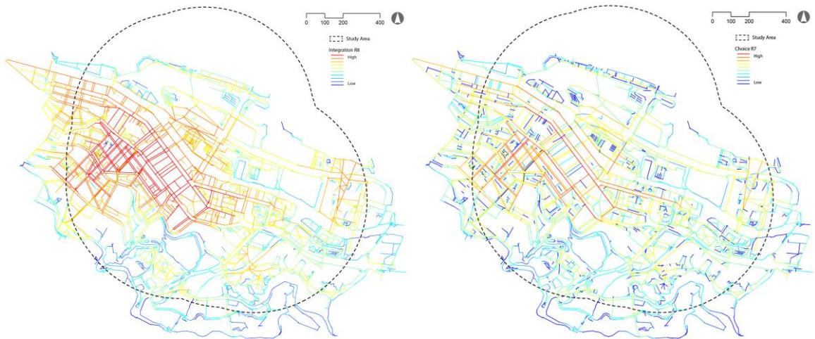
Figure 5. Closeness (Integratin at Radius 8) and betweenness (Choice at Radius 7) of axial map in Central area, warmer lines are closer to other lines and more central.
